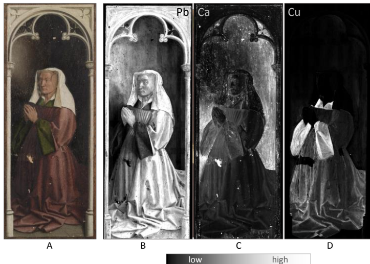
Fig. 1. The panel 'Elisabeth Borluut' (A) and several elemental distributions obtained by means of MA-XRF (University of Antwerp): lead (B), calcium (C) en copper (D). In the copper distribution, the small area where the overpaint layer was removed is clearly visible.
