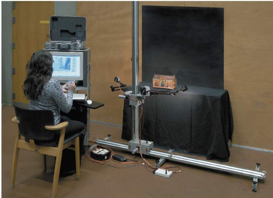
1. Infrared reflectography (IRR) with a platinum silicide focal plane array video camera, mounted on a Scannix remote controlled rail system.
