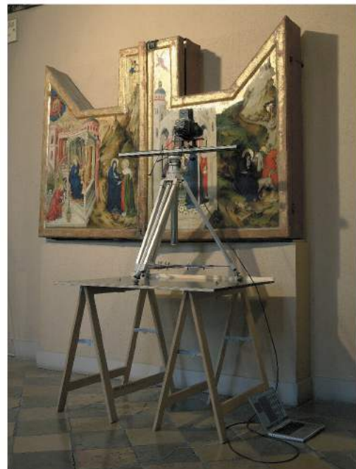
3. Digital infrared photography (IR) with a Phase One LightPhase camera, mounted on a manually operated rail on a Linhof tripod.
